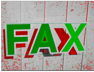
Fig. 16 Illustration of texture-based validation process: validated hypothesis are blue boxes, rejected hypothesis are red boxes.
